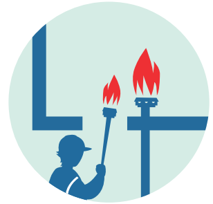
Check atmosphere in Fire box before igniting the burners
